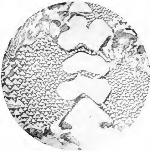
A. Alloy of antimony and \text{Cu}_2\text{Sb} . \times 200 .
